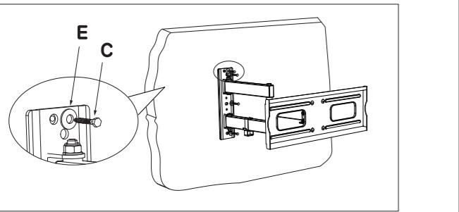
**2** Install the support on the wall using four bolts and four metal washers.
