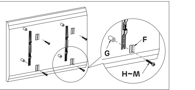
**3** Install the brackets on the TV's backside. Use two bolts and two square metal washers in each bracket. The bolts should be selected according with the dimensions of the holes. Use the spacers if needed.
