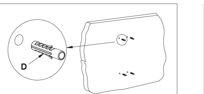
**1** Use the support's wall plate as a template to mark four holes. If it is a concrete wall, the holes should have 10 mm in diameter and 50 mm in depth. Wedge the four plastic anchors into the drilled holes.
